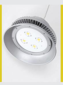
lightweight cast aluminium body plays a role in radiating heat as well as light, making Atena ideal for larger spaces such as school halls and gymnasiums. Powder coated in grey. Power options available: 15000 lm (129W power), 20000 lm (172W) or 25000 lm (215W). Colour temperature of LED sources: 5000K. Dust and water resistant to IP65 standards, guaranteeing long term performance and reliability.
